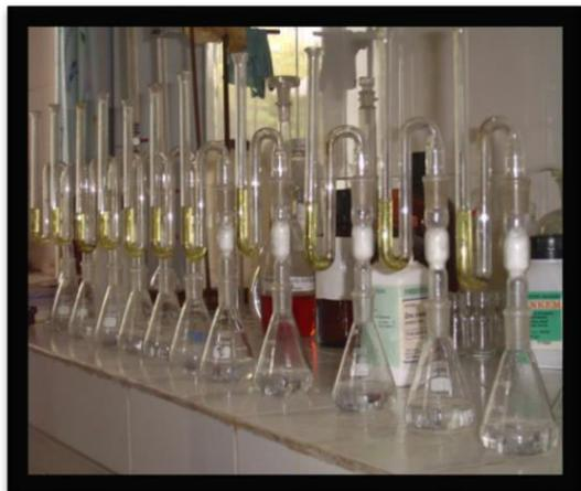
**Fig -1:** Arsenic concentration testing
